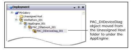
4 Check out and edit the new object so it can be configured. As with all ArchestrA instances, double-click on the object to check it out from the Galaxy and open it. The DIDevice configuration window opens, with the **General** tab displayed.
