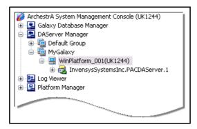
**4** Expand the appropriate DAServer (InvensysSystemsInc.PACDAServer.1 in the example) to reveal the Configuration and Diagnostics folders.
