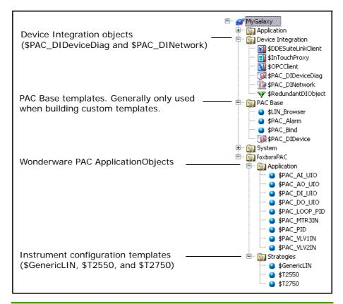
**Note:** The \$PAC\_DIDevice template is located within the PAC Base folder tree. Use the \$PAC\_DIDevice instance to communicate with non-Foxboro PAC instruments (that is, instruments other than the T2550 and the T2750). For T2550 and T2750 instruments, the use of a \$PAC\_DIDeviceDiag instance (under the Device Integration folder tree) is recommended.
