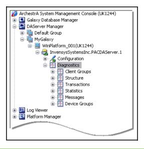
**Important:** Do not make any changes to the settings within the Configuration folder. Unpredictable results may occur. Only make configuration changes to the PAC DAServer using the IDE.
