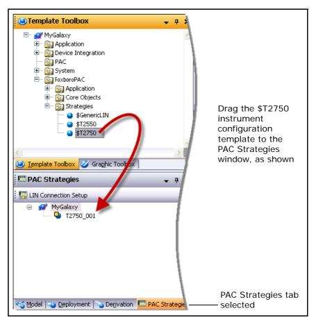
The default name for the new instrument configuration is T2750\_nnn, where nnn is a sequential number starting from 001. The PAC instrument can be renamed in the usual manner within ArchestrA, if required.
