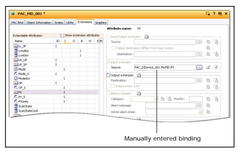
The binding of the PAC instrument's PV value to the ArchestrA PID object is complete. The object can now be checked back in. In order to check the binding, the Object Viewer utility can be opened and the PAC\_PID\_001.PV can be added as an Attribute Reference to a Watch window. If the configuration is correct, the live PV value is displayed. For information on the Object Viewer utility, see the *Object Viewer User's Guide*.
