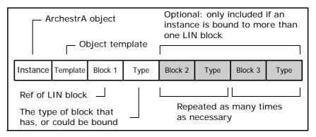
If an ApplicationObject is bound to multiple LIN blocks, then the last two fields (**Block n** and **Type**) are repeated as many times as necessary. The ApplicationObject configuration is regarded as complete when the line ends.
